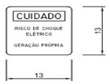
PLACA EM AÇO INOXIDÁVEL OU ALUMÍNIO ANODIZADO, COM ESPESSURA MÍNIMA DE ÍMM, FUNDO AMARELO E FONTE PRETA. A FIXAÇÃO DEVE SER FEITA COM PARAFUSOS OU REBITES. COTAS EM CENTÍMETROS.
